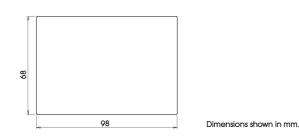
Before cutting the hole, ensure that enough room is available within the dash for the area of the module and the Securing Bracket. Access to the back of the dash will be required to secure the Sigmagauge.
