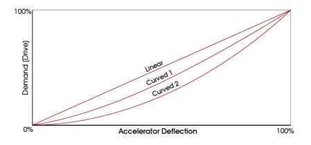
This sets the type of response for both the Accelerator and Footbrake inputs (pins 8 & 9 on Connector A). There are three options for Permanent Magnet Traction control, Linear, Curved1 and Curved2.
